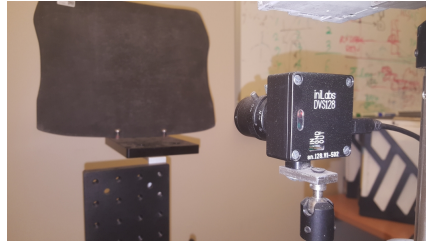
Figure 3.5. DVS128 sensor used in our experiment for data collection. In each data collection experiment, the sensor was kept under constant illumination in an empty room isolated from any activity.
