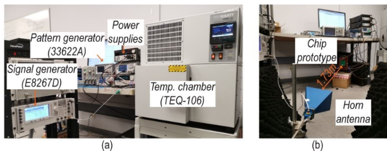
Figure 3.16. Photos of (a) across temperature test setup, and (b) wireless test setup.
