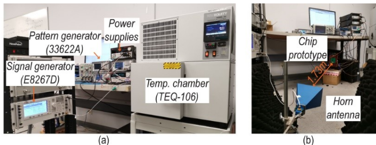
Figure 3.16. Photos of (a) cross temperature test setup, and (b) wireless test setup.
