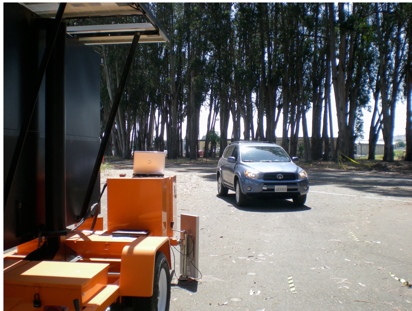
Figure 5. RFID Reader At the Entrance of BART Lafayette Station Parking Lot
