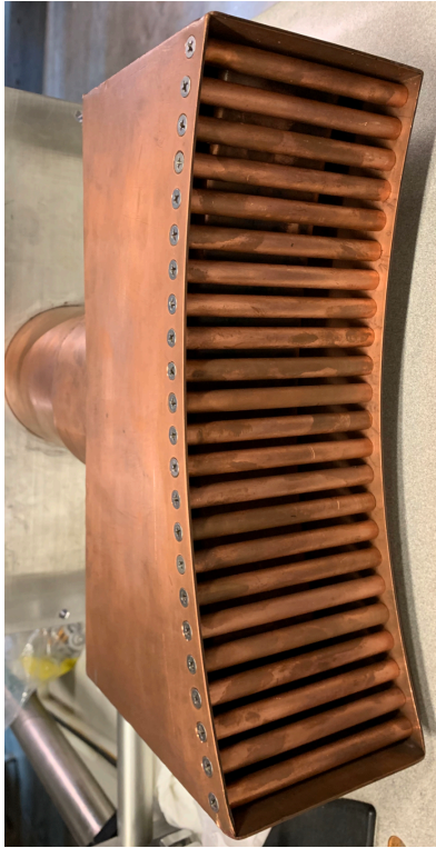
Figure 6.1: Single-Strap RF Antenna with Faraday Screen
