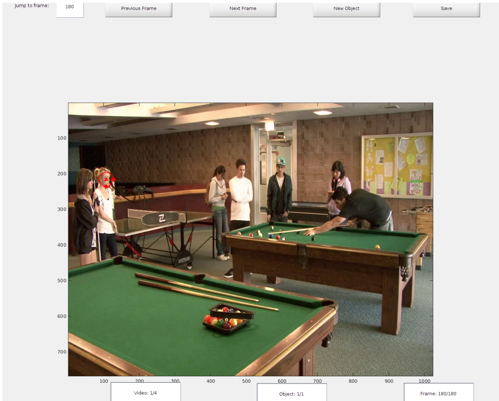
Figure 3.2: A snapshot of the custom face annotation tool in Matlab. This provides an easy way to draw ellipses to fit the shape of faces. In the above image, the ellipse is initialized on a person’s face (red region on the left) and resized by the annotator accordingly to fit the face.
