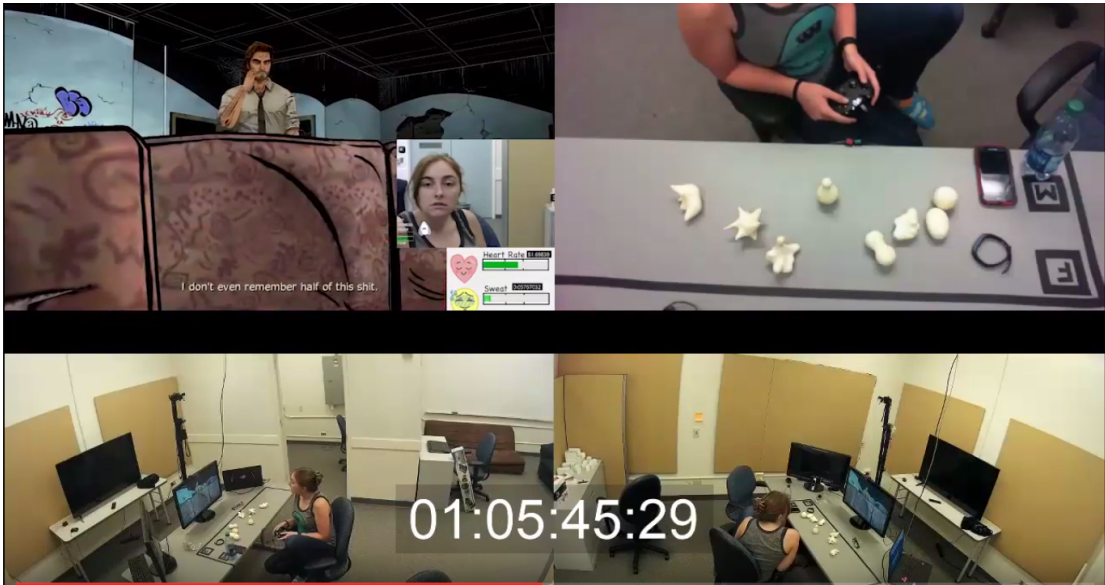
Figure 3.4: Lab setup including biometrics, SEI, and 4 cameras. Upper left is front-facing webcam, upper right is top-down webcam focused on the SEI, and lower left and right parts are the left and right room webcams respectively.
