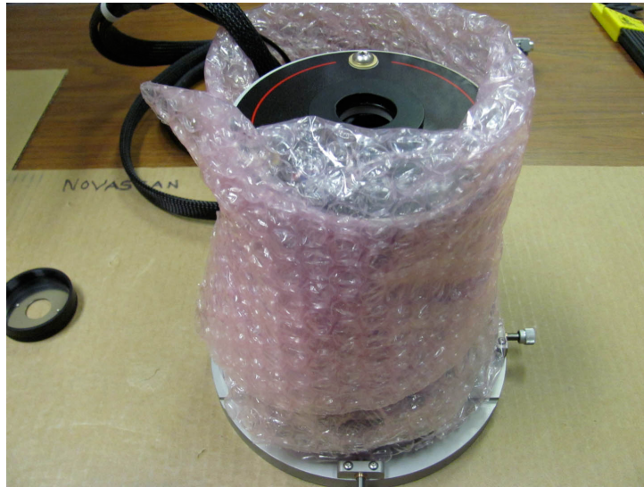
Figure A1. 19 Wrap the AFM head with anti-static bubble wrap; with the cables oriented to the top of the AFM head.
