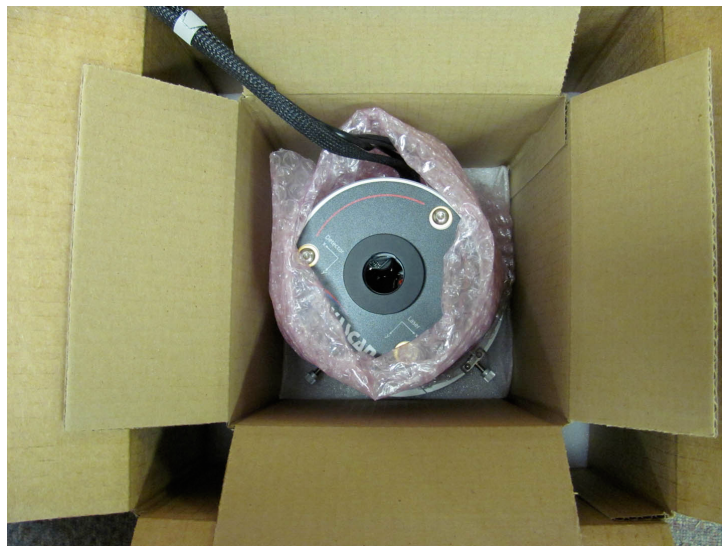
Figure A1. 20 Place the wrapped AFM into the inner packing box with foam at the bottom, make sure to have translation screws are oriented to the corners of the box.
