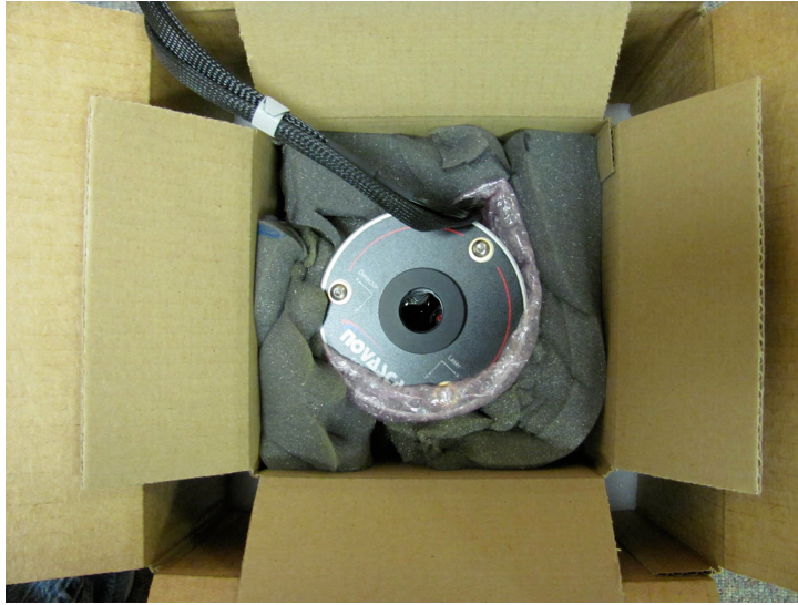
Figure A1. 21 Pack more foam around AFM head inside of inner packing box
