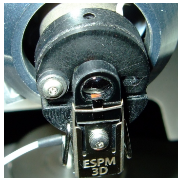
Figure A1. 3 Image of the probe holder with the probe underneath, the probe holder is still attached to the scanner; the probes can be taken out or put in simply by pressing down the letters ‘ESPM 3D’ while the probe holder installed to the platform which holds the probe holder for probe switching.
