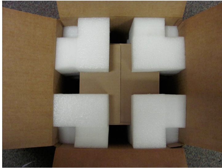
Figure A1. 23 Add foam protectors between the inner packing box and outer packing box.
