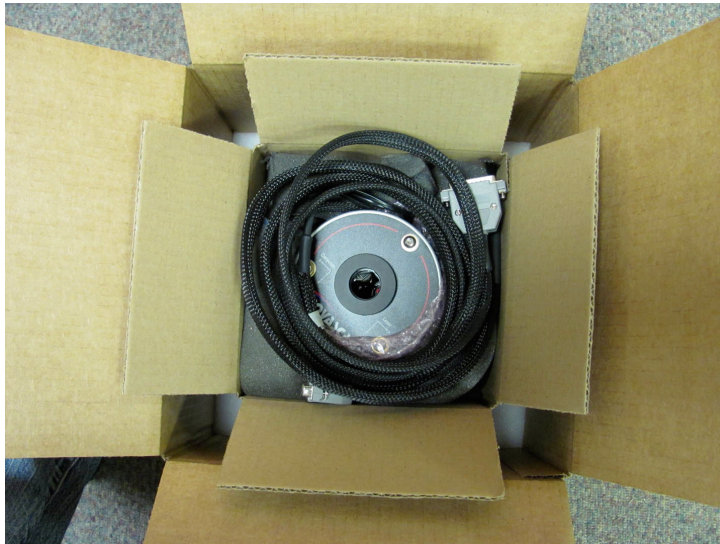
Figure A1. 22 Coil the AFM cables and place them on top of AFM head
