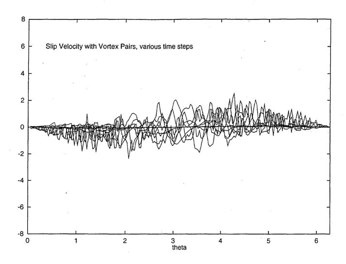
Fig. 4 Using Coupled Vortex pairs in the interior, vortex sheet near the boundary. The slip velocity over the cylinder for time steps 8, 9 and 10
