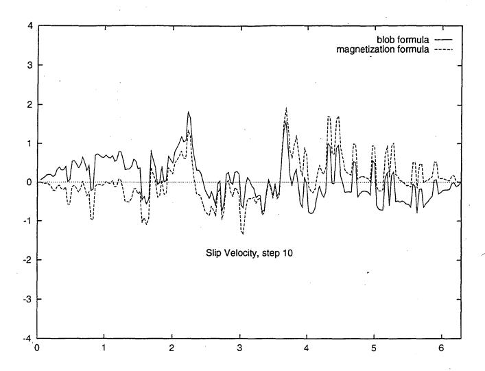
Fig. 3 Using magnetization variables (but with vortex blob information carried also) in the interior. Vortex sheets are used near the boundary. No magnet strength evolution. Tangential velocity on cylinder at step 10 — the 'slip' to be extinguished during next time step — evaluated using 1.) magnetization formula, or 2.) Biot-savart formula
