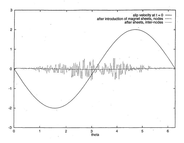
Fig.2 No slip established after introduction of "sheet magnetization" at t=0, evaluated at the nodes of integration, and at mid-points of integration interval
