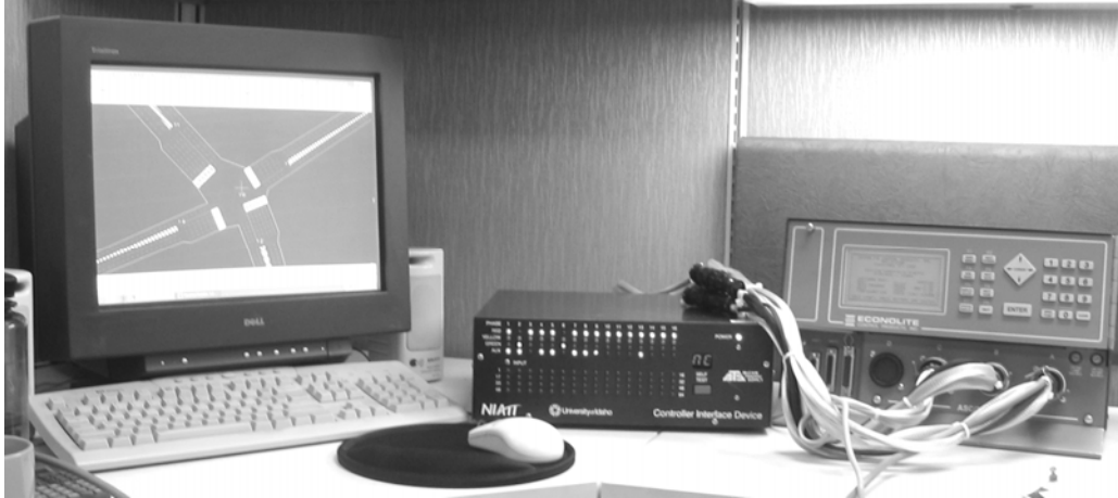
Figure 2.12: Connectivity between CID-II, Paramics and NEMA Controller
