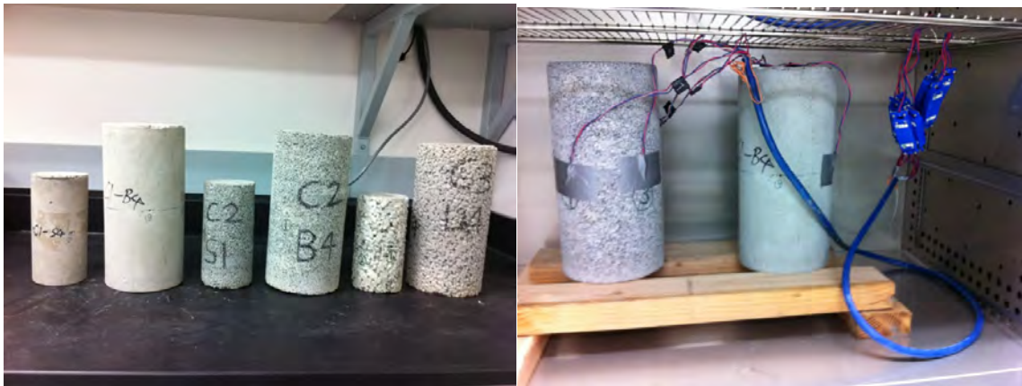
Figure 6.14. Example concrete specimens used for testing and test setup.
