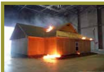
Photo 2. In order to be effective, external sprinklers must be able to wet all areas where ignition can occur, or be sufficiently effective in quenching embers that approach the home so they won't have enough energy to ignite combustible items.
