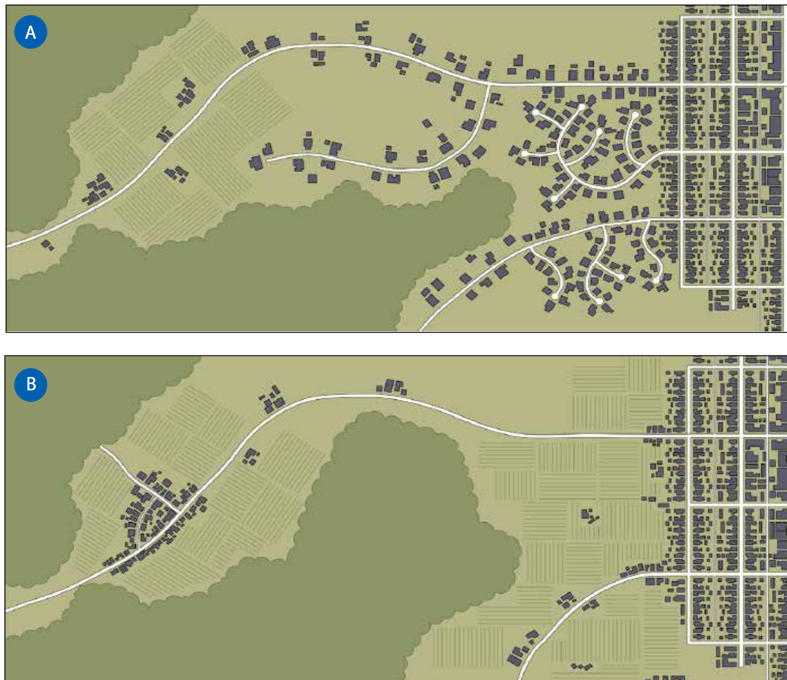
Figure 8. Comparison of conventional versus clustered development employing a protective agricultural buffer. A scattered pattern of conventional suburban sprawl (A) often transforms agricultural land (shown as striped rows) as development expands from a residential core (dense community on right). This development pattern requires greater area in “zones of defense” (light color) and thus more clearing of native vegetation (dark color); the more diffuse spacing of homes also requires more firefighting resources and makes fire suppression more complex.
