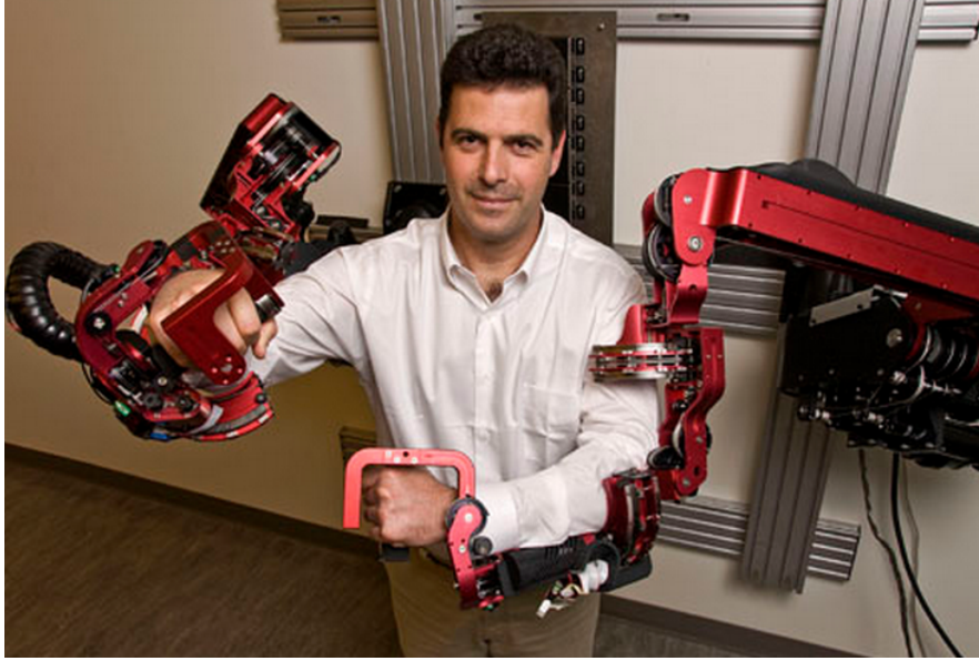
Figure 1.2: The 7-DOF EXO-UL7 upper limb robotic exoskeleton device [73].
