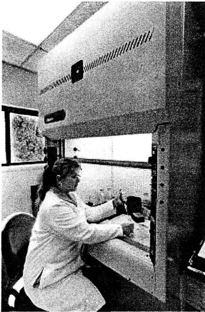
Figure 2. Berkeley fume hood.
