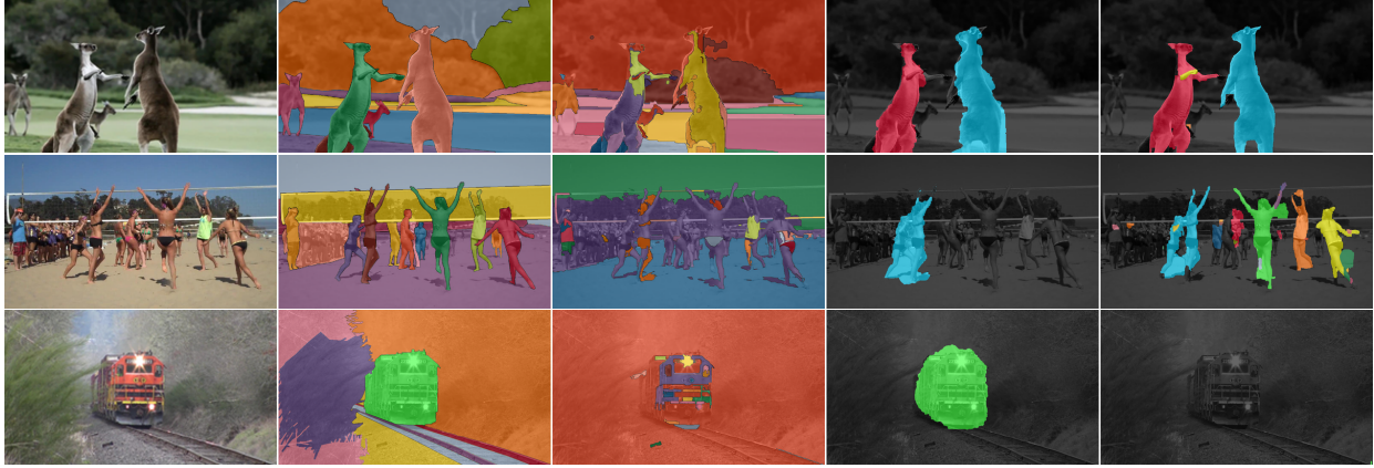
Figure 2.12: Sample results on BVSD. Left to right: original image, ground truth, [GKH10],[OMB14], ours (object maps). Row 1: as reflected by BPR, our method produces accurate boundaries (see Fig. 2.9). Both actors are correctly segmented—the arm occluding the animal’s body is a distinct depth layer. Row 2: “failure case”—complex motion and inaccurate flow can result in inaccurate segmentations. Row 3: failure case—object is not detected throughout the sequence due to lack of occlusions.
