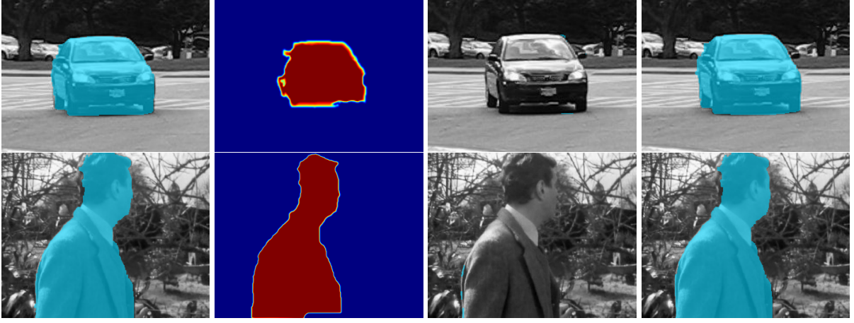
Figure 2.4: c_{t-1} (column 1) is used to compute the foreground prior ( \kappa_t ) (column 2). Without \kappa_t , the resulting c_t completely misses the objects (column 3), however with \kappa_t , c_t succeeds (last column). Note c_{t-1} and c_t look very similar— \kappa_t helps most during small-baseline motion when occlusion cues are weak but c_{t-1} easily predicts c_t .
