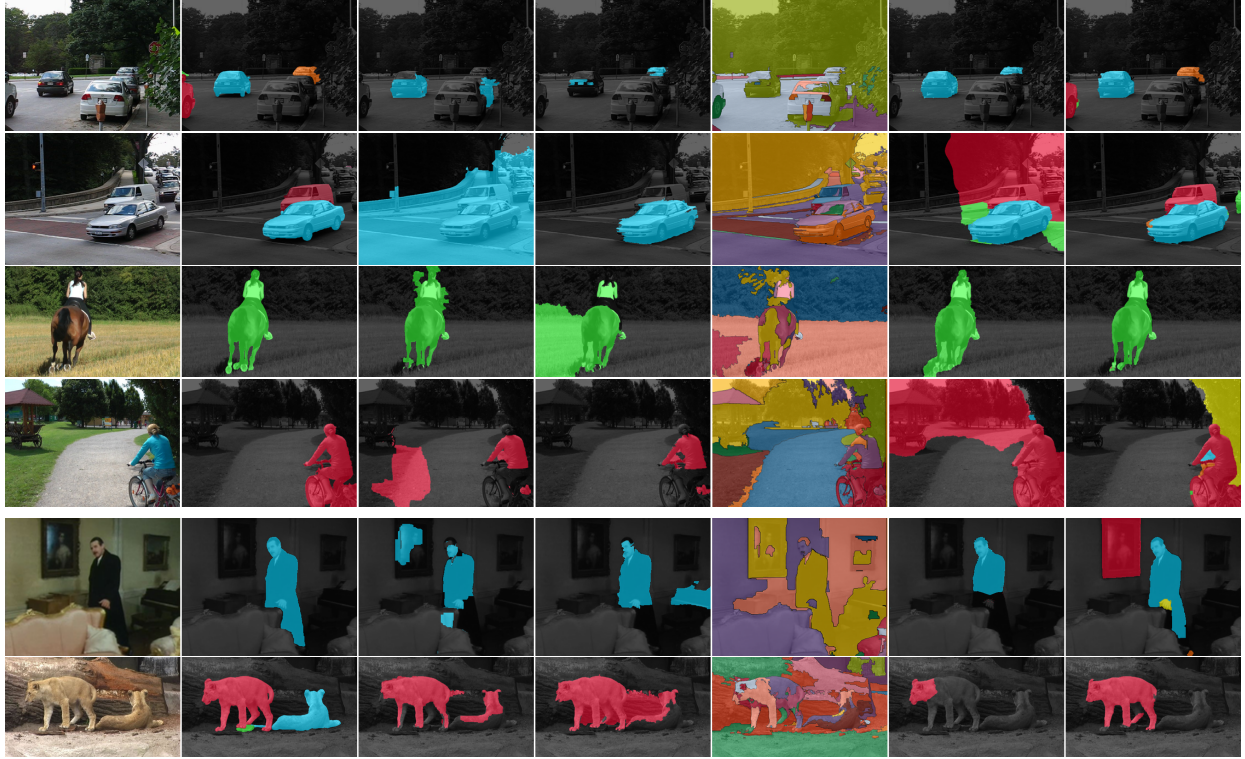
Figure 2.13: Sample results on MoSeg. Left to right: original image, ground truth, [LKG11], [PF13], [GKH10], [OMB14], ours (object maps). Top two rows: occlusion cues allow us to obtain even the barely visible cars (row 1 - orange, row 2 - red, row 2 - green). Row 3: use of both motion and appearance cues allows us to generate an accurate object boundary. Row 4: occlusion cues yield three depth layers (bicyclist, tree, background) (see also Fig. 2.1). Notice that the tree (and some cars in rows 1–2) is not annotated, so our scheme is penalized despite providing the correct answer. [LKG11, PF13] suffer from trailing and only produce binary segmentation. [GKH10] suffers from oversegmentation. [OMB14] performs comparably to our method; The last two rows show failure cases. Row 5: the painting is recognized as an “object” due to false occlusion detection; the hand is assigned to a separate layer. Row 6: the lioness is missed due to insufficient motion and lack of occlusions.
