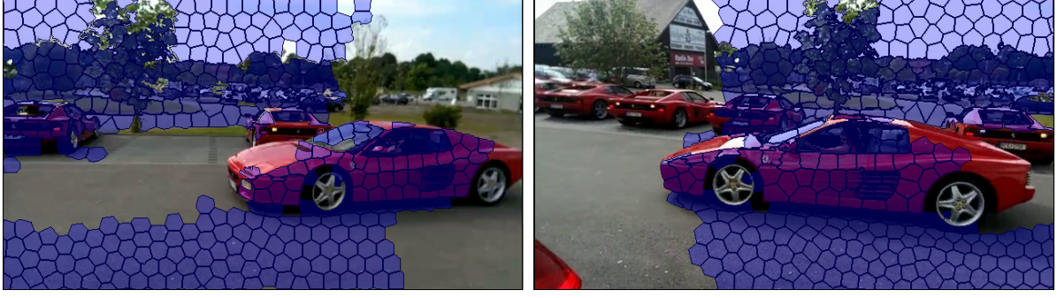
Figure 3.2: A pair of frames with temporally consistent regions ( \{S_i\} , [CWI13]). The highlighted regions are present in both frames.
