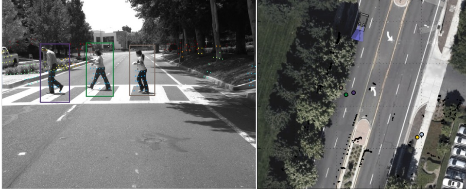
Figure 5.4: Left: Sample frames from the front camera, with LiDAR returns (colored by depth) and the detected pedestrians. Right: Bird's-eye-view of the scene. The vehicle is in north-west corner and pedestrians, shown by circles, are in the center. LiDAR returns are shown in black. Note that the satellite image is outdated and does not contain the pedestrian crossing seen in the images.
