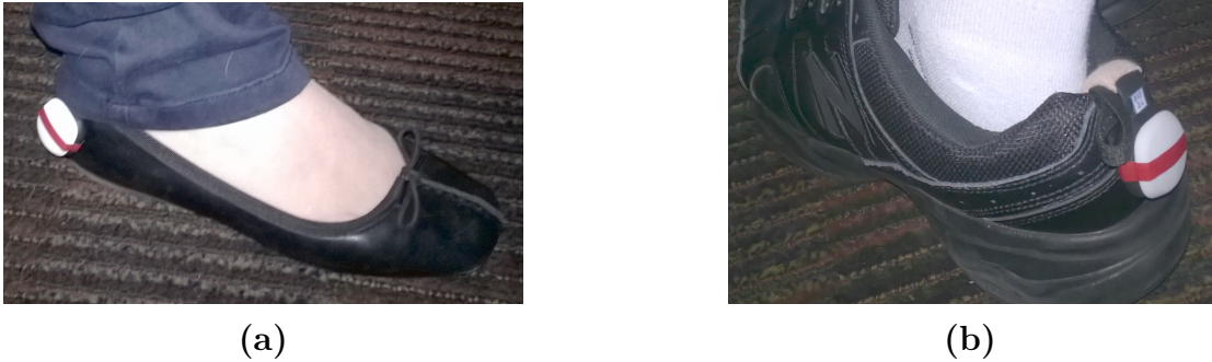
Figure 3.1: Examples of placement of the CPRO shoe-mounted sensor for ground truth step detection. The sensor is contained in the white small case, attached to a plastic padded clip, and clipped to the back of the shoe.
