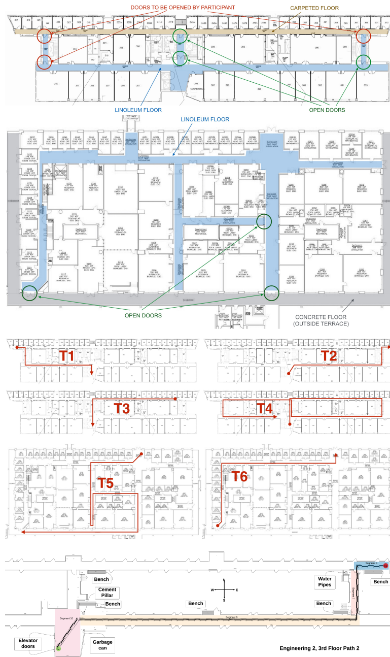
Figure 3.3: Top two rows: the floor plans of E2 and BE, respectively. Third row: the trajectories taken by our participants. T1-T4 were located in E2, T5-T6 in BE. Fourth row: Detailed annotated map of trajectory T2 walked by the participants.
