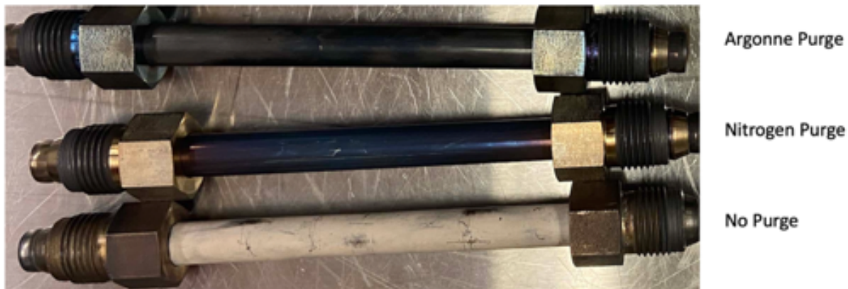
Figure 8-2: Effect of furnace atmosphere on test sample oxidation.
