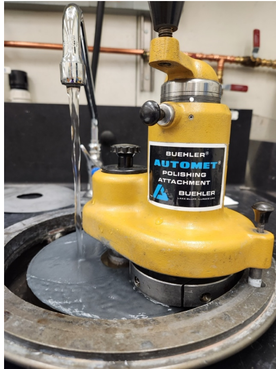
Figure 3-7: Grinding samples on SiC paper with water lubricant.
