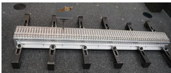
Figure 3: Clamped magnet module.
