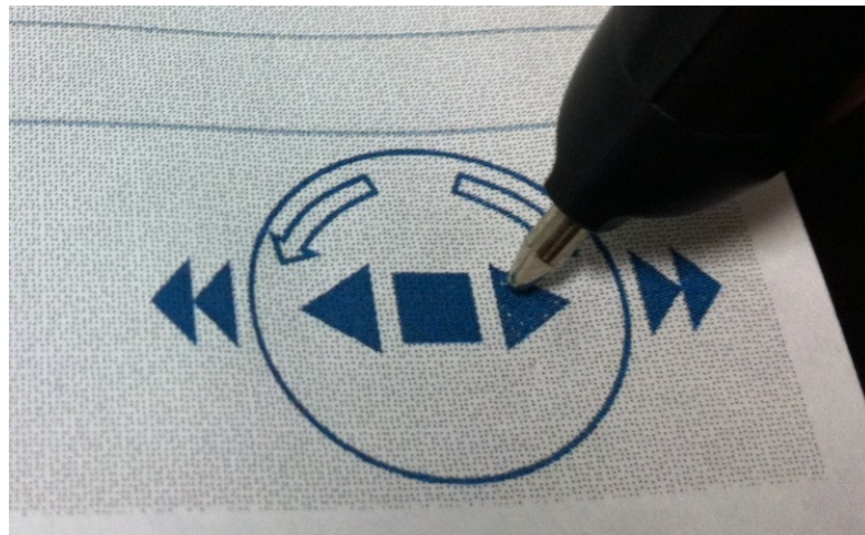
Figure 4.6: Video playback controls printed on Anoto paper. A user can tap on the controls with a Bluetooth Anoto pen to control video playback in ChronoViz.
