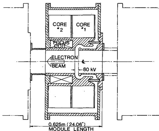
Fig. 3. Schematic of one of the 64 accelerator modules.
