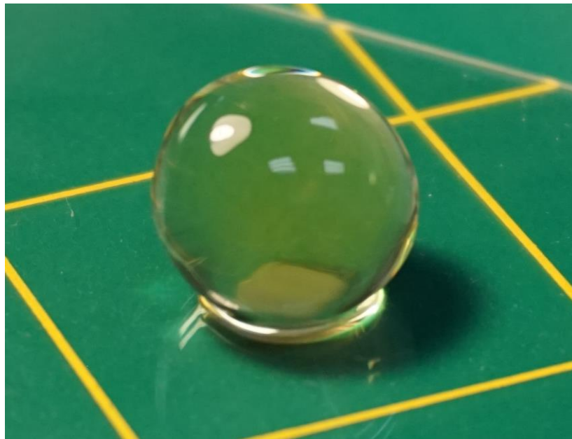
Figure 4-18 Smooth sphere printed in gelatin methacrylate with no layer lines.
