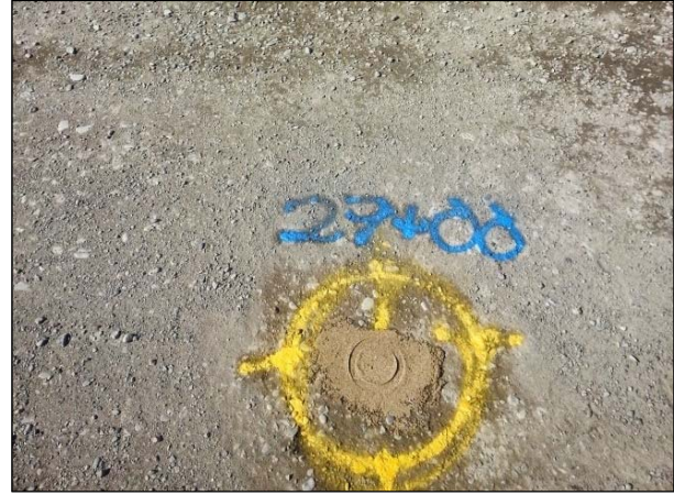
Figure 2.14: SSG footprint in sand patch.
