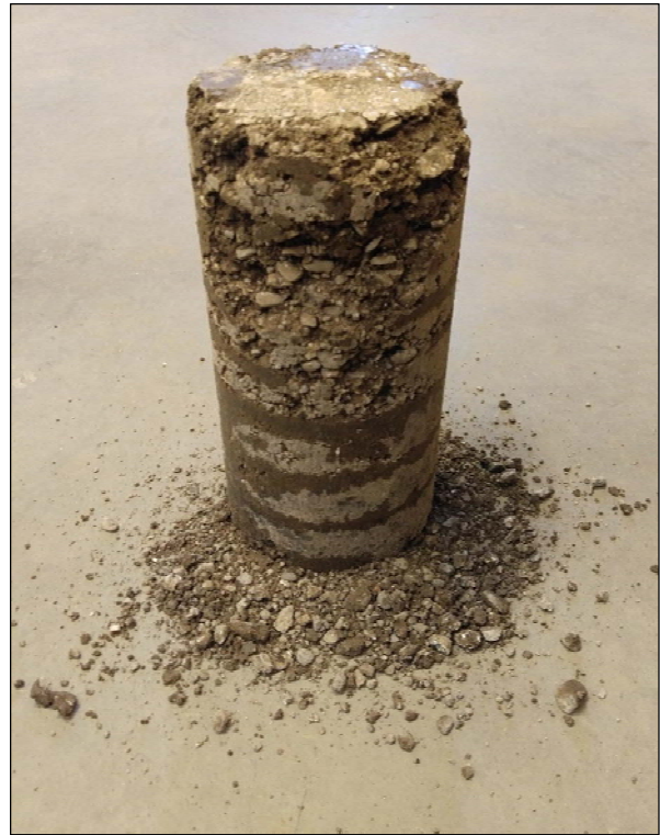
Figure 5.2: Result of microcracking effort with vibrating hammer.
