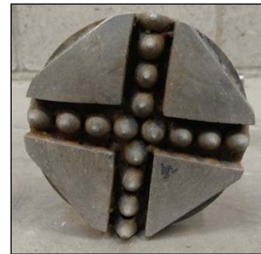
Figure 6.5: Scouring tool: general view and bottom view.
