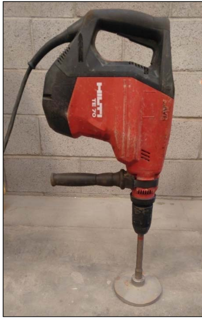
Figure 6.4: Vibrating compaction hammer with 148 mm compaction attachment.
