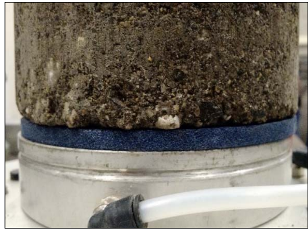
Figure 6.15: Irregular specimen ends leading to poor contact.
