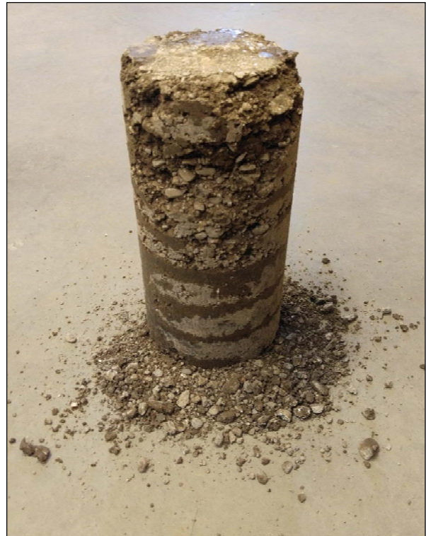
Figure 5.2: Result of microcracking effort with vibrating hammer.
