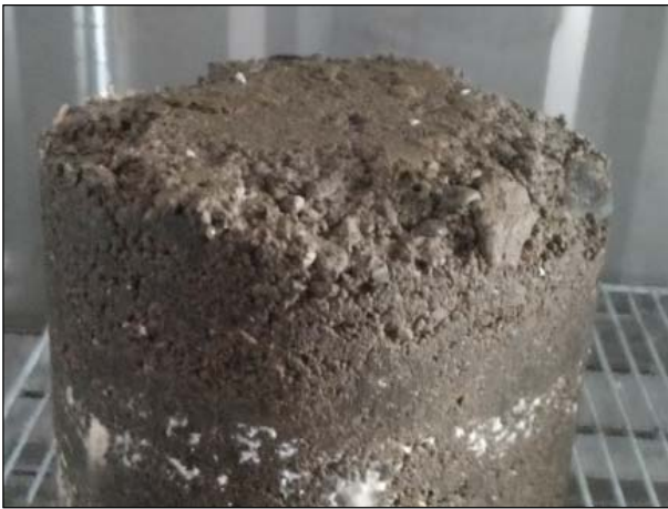
Figure 6.14: Broken edges caused by brittle nature of stabilized material.
