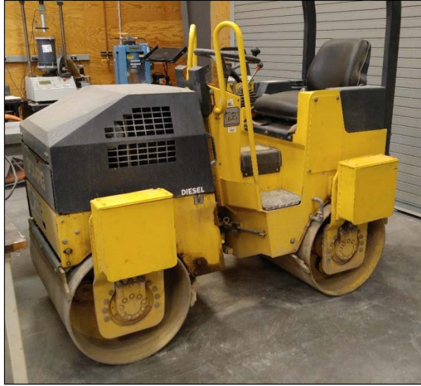
Figure 5.4: Steel wheel vibrating roller.
