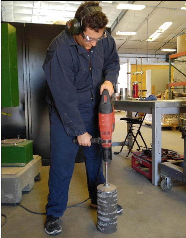
Figure 5.1: Using the vibrating hammer to microcrack a compacted specimen.
