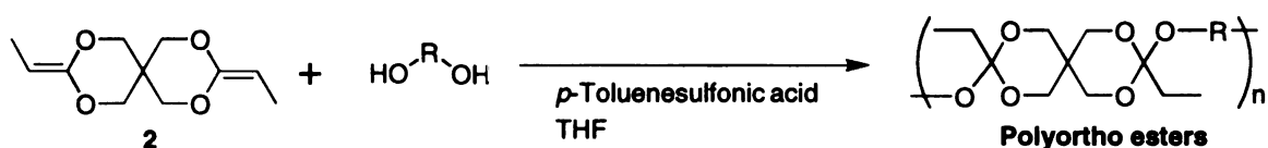
Scheme 4-1: Synthesis of polyortho esters using 3,9-diethylidene-2,4,8,10-tetraoxaspiro[5.5]undecane and diols in the presence of an organic acid catalyst.
