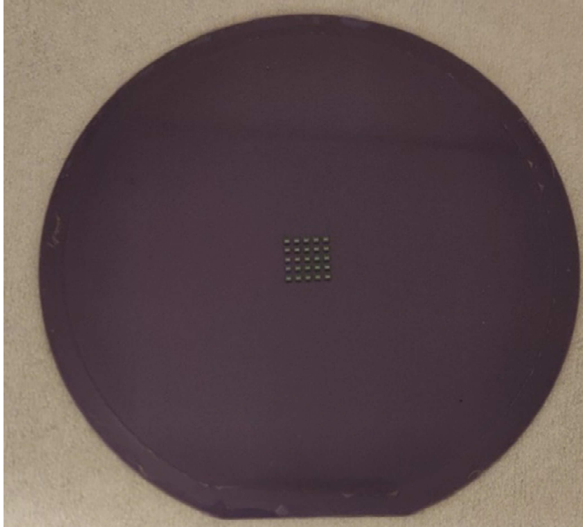
Figure 4. 21. The image of the sample with 5 x 5 array of dies received by UCLA.
