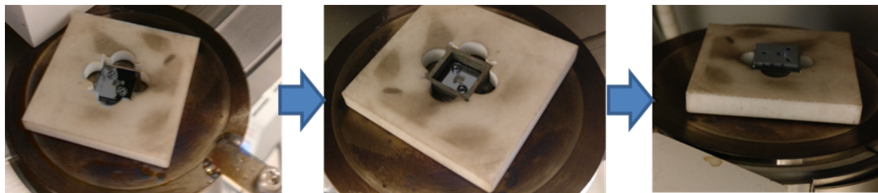
Figure B.6: sample loading sequence: loading sample on the lower electrode then putting the ceramic frame, putting the metallic frame, putting dummy silicon sample to make the stack taller than the ceramic frame, returning the lower electrode to its position.
