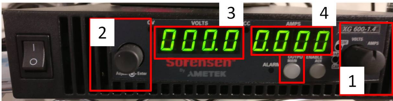
Figure B.9: High Voltage supply interface showing: 1) voltage or current selection knob, 2) adjustment knob, 3) Voltage reading, 4) current reading, and the main output toggle button)
