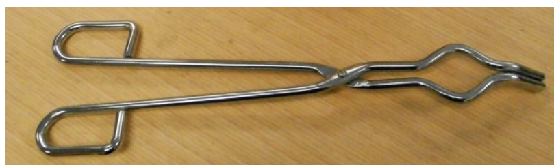
Figure B.3: Clamp to carry hot boat.
