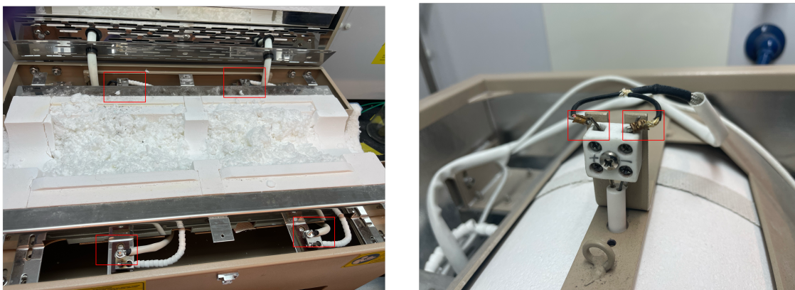
Figure 2.4: MTI two-zone furnace Left: Interior of the tube furnace, showing the measurement points used to verify heating elements' resistance with a multimeter (highlighted in red). Right: Access panel to the thermocouples; the regions highlighted in red indicate the locations where resistance measurements are performed using a multimeter.
