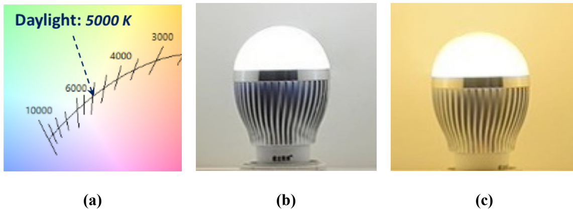
Figure 1.6 (a) The CCT value of warm and cool white (from 2500 to 10000 K) and the CCT value of daylight (pointed) in the CIE diagram [17]. Photographs of (b) cool white LED and (c) warm white LED [19].
