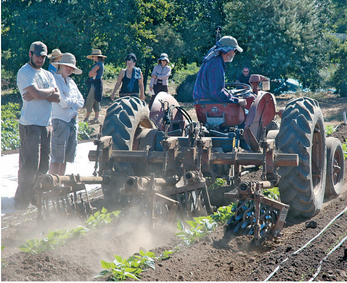
FIGURE 6. A rolling cultivator re-forms planting beds and “dirts” growing beans, burying the drip lines and any weeds.
