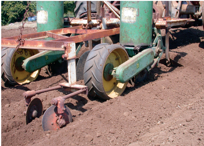
FIGURE 4. Disc hillers create a soil cap over the seed line. Photo: Jim Leap
