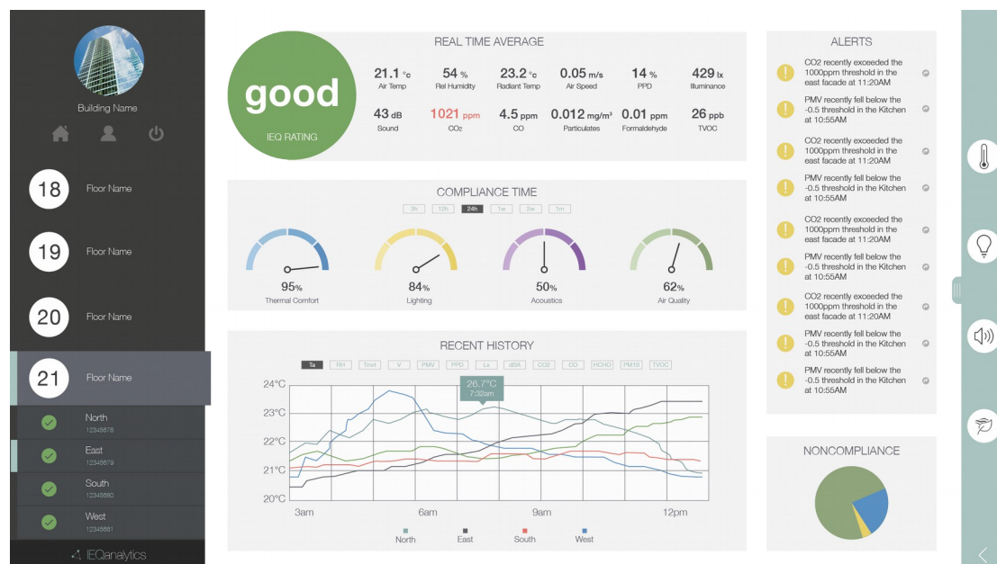
Figure 5. A mock-up of the IEQAnalytics dashboard, as seen by end-users of the service. Devices on different floors of the building may be selected through the left-
