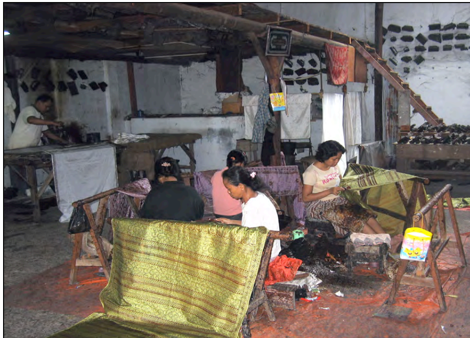
Fig. 89. Batik factory, Trusmi, Cirebon. 2006. Today, women do the exacting work of hand drawn batik ( tulisan ) in very close proximity to each other. Positioned in the center, is a collective pot of hot wax that the women draw from. Notice the one male worker in the far left rear. Batik stamps adorn the rear walls.
