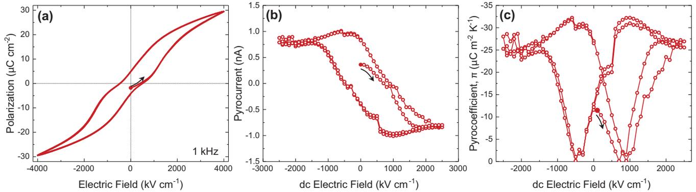
FIG. 2. (a) Polarization-electric field hysteresis loop measurements showing a pinched or constricted hysteresis loop in the as-received Si:HfO<sub>2</sub> films. (b) Pyroelectric current ( $i_p$ ) and (c) pyrocoefficient ( $\pi$ ) measured as a function of background dc electric field, at 1 kHz. The black arrows and filled red data point show the direction and starting point of the measurements.
