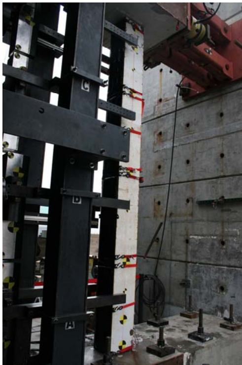
Figure 5.49: Test WA05 with Water Bladders
