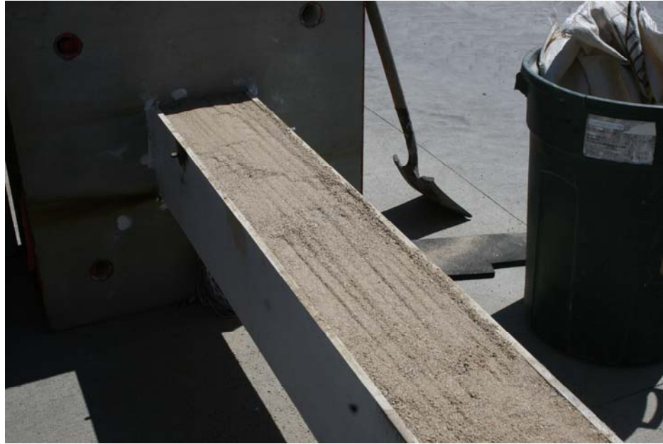
Figure 5.16: Column Laid Horizontally and Filled with Sand
