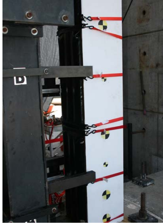
Figure 5.28: Test WA02 Column with Water Bladders Attached
