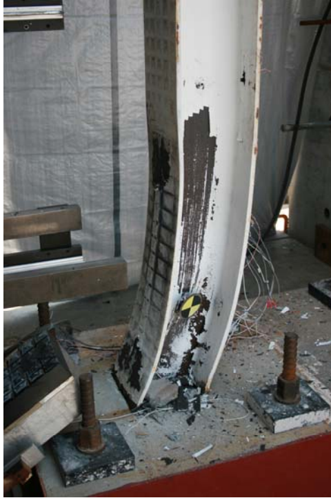
Figure 3.67: Test SA11 Column Base Post-Test (View 1)
