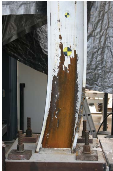
Figure 3.60: Test SA10 Column Base Post-Test
