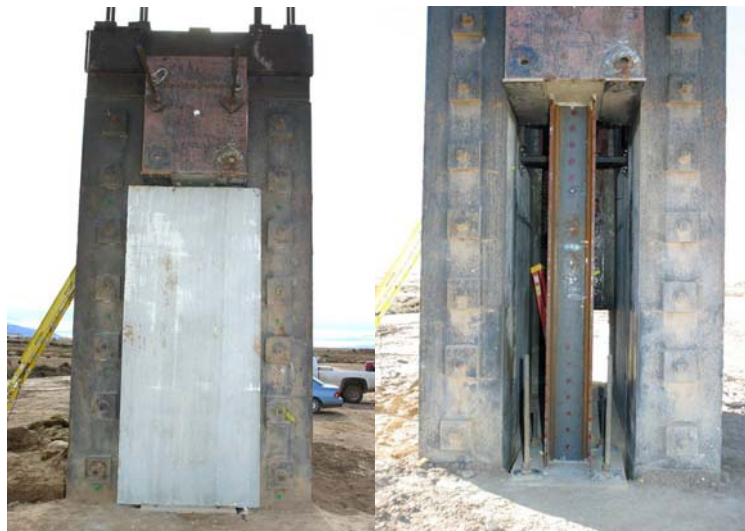
Figure 2.14: Field Tests, Phase I With (left) and Without (right) Concrete Cladding
