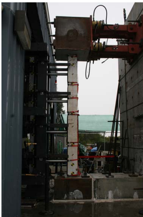
Figure 5.50: Test WA05 Column Pre-Test
