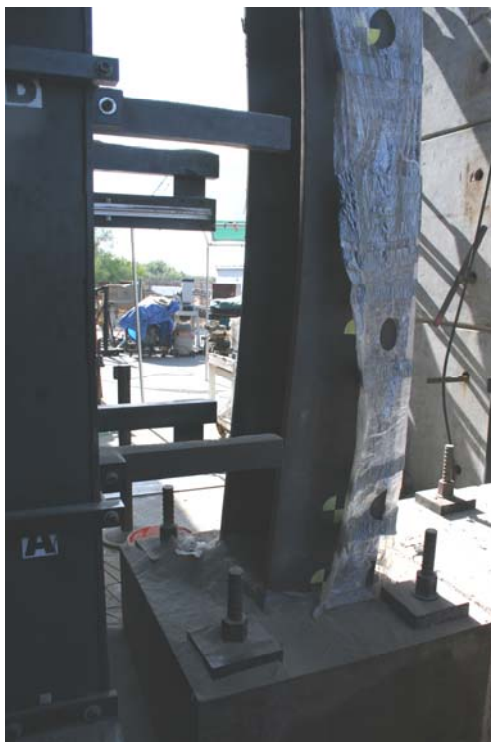
Figure 5.47: Test WA04 Column Base Post-Test
