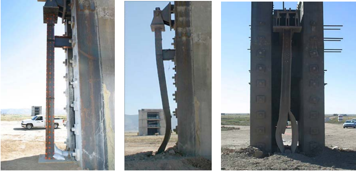
Figure 2.17: Before and After Photos from Test 10 without Cladding
