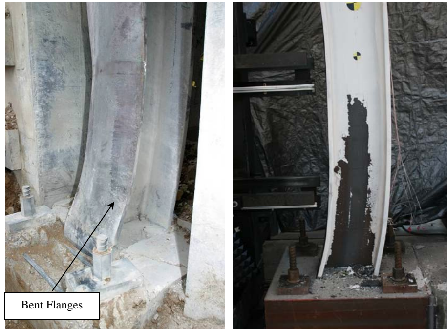
Figure 3.74: Flange Behavior Comparison of Field Test (left) to Simulator Test (right)
