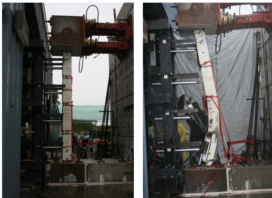
Figure 5.70: WA05 Pre and Post-Test Global Deformation
