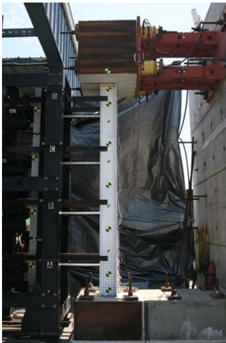
Figure 3.27: Test SA01 Column Pre-Test
