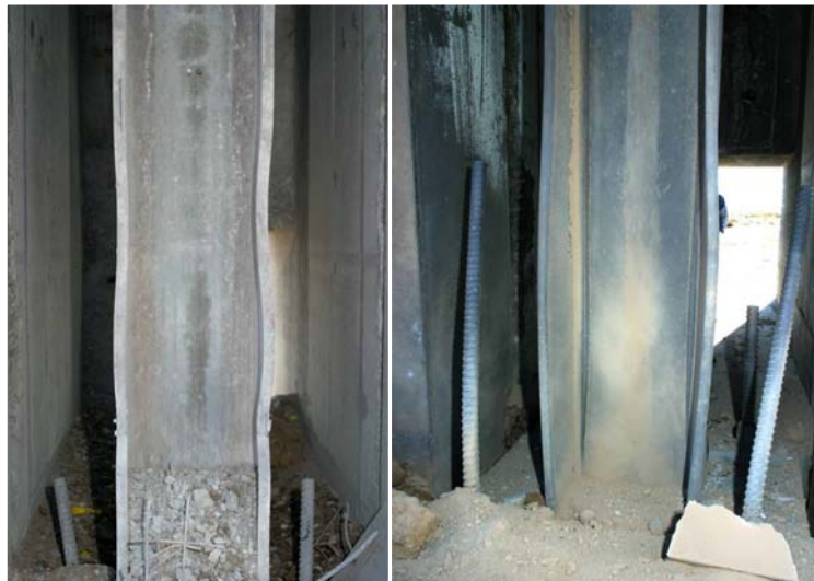
Figure 2.15: Comparison of Tests With (left) and Without (right) Cladding
