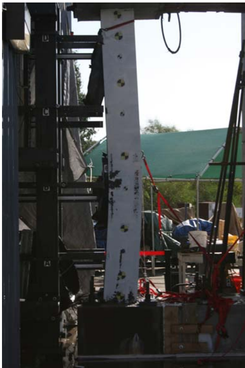
Figure 5.39: Test WA03 Column Post-Test
