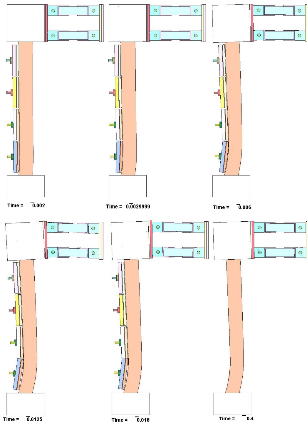
Figure 4.41: Test SA07 Finite Element Run Progression
