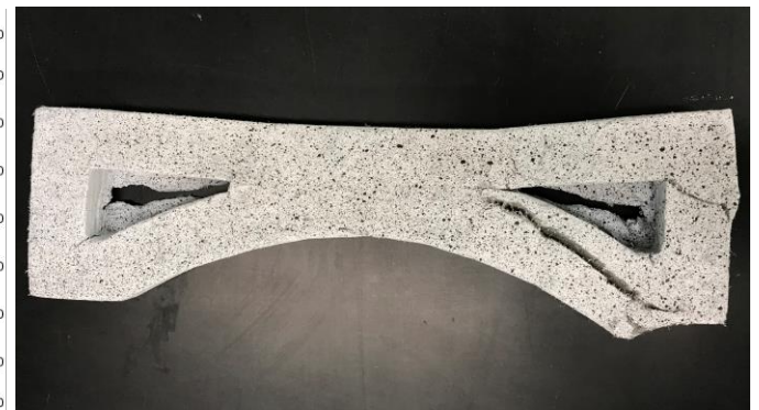
Figure 97: Image of damage pattern in Specimen CL 3D-8 after four-point bending test
