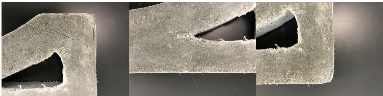
Figure 60: Microcracks formed around the corners (notches) due to stress concentration
