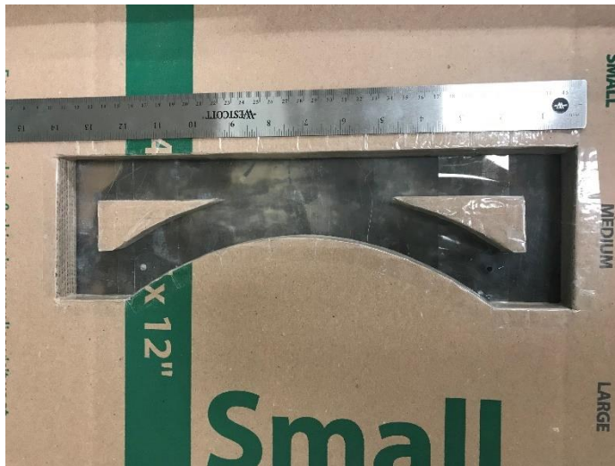
Figure 44: Cardboard mold for the topology optimized beam with length measurement
