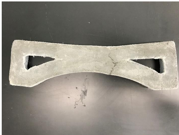
Figure 57: 3D printed topology-optimized beam (Specimen 3D-2) after testing
