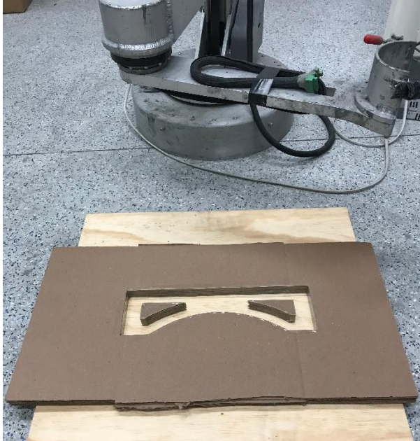
Figure 47: 3D printing of topology-optimized beam with a SCARA robot
