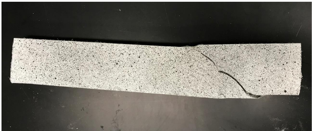
Figure 114: Final failure crack in Specimen CL PE-5 indicating shear-governed failure
