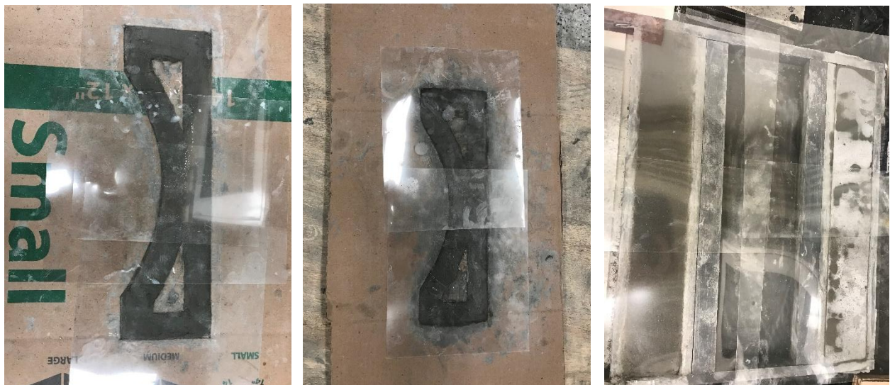
Figure 50: Fresh specimens covered with plastic sheets for curing for the initial four days
