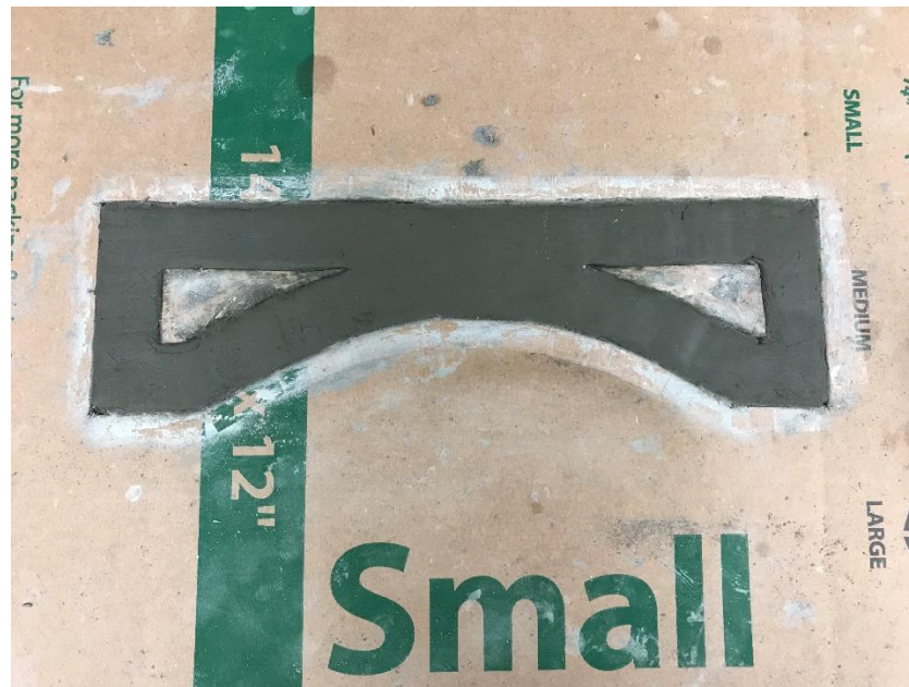
Figure 46: Casted beam with optimized topology
