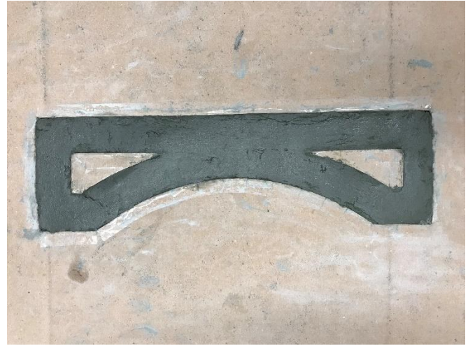
Figure 48: 3D printed beam with optimized topology made of high-strength ductile concrete
