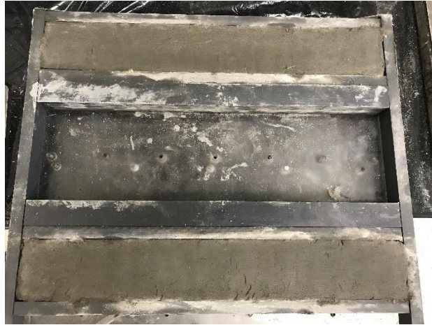
Figure 49: Casted prismatic beams made of high-strength ductile concrete
