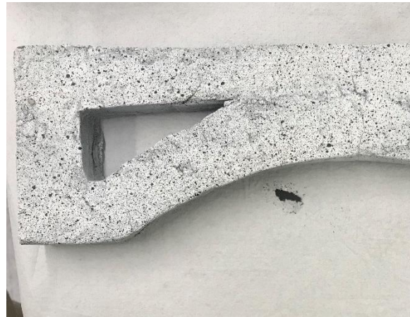
Figure 52: Specimen spray-painted with a black dotted pattern for subsequent DIC measurement of strain field
