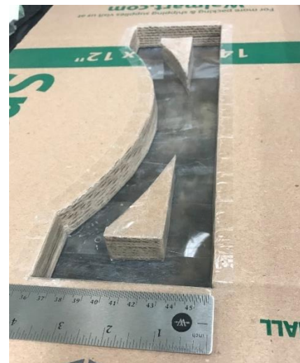
Figure 45: Cardboard mold for the topology optimized beam with side measurement
