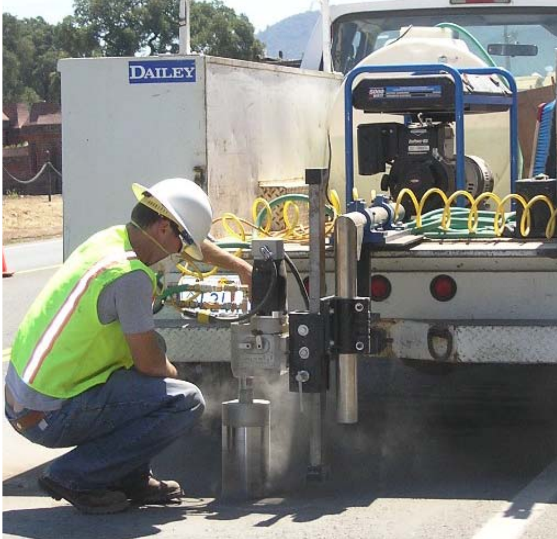
Figure 3-5. Equipment for taking dry cores in the field.
