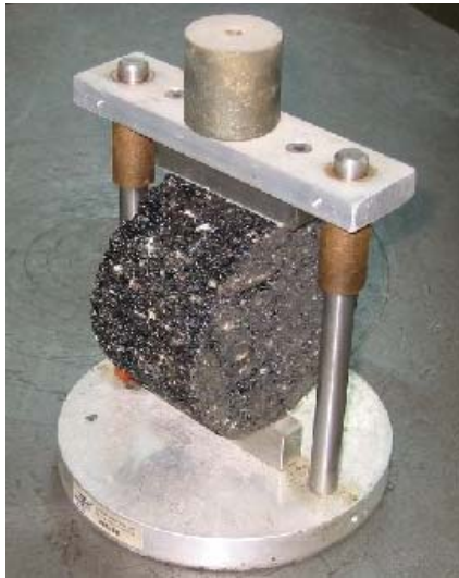
Figure 6-13. Equipment used for the TSR test (a – Southwark Tate-Emery hydraulic testing machine, b –Gilson MS-35 Lottman breaking head).
