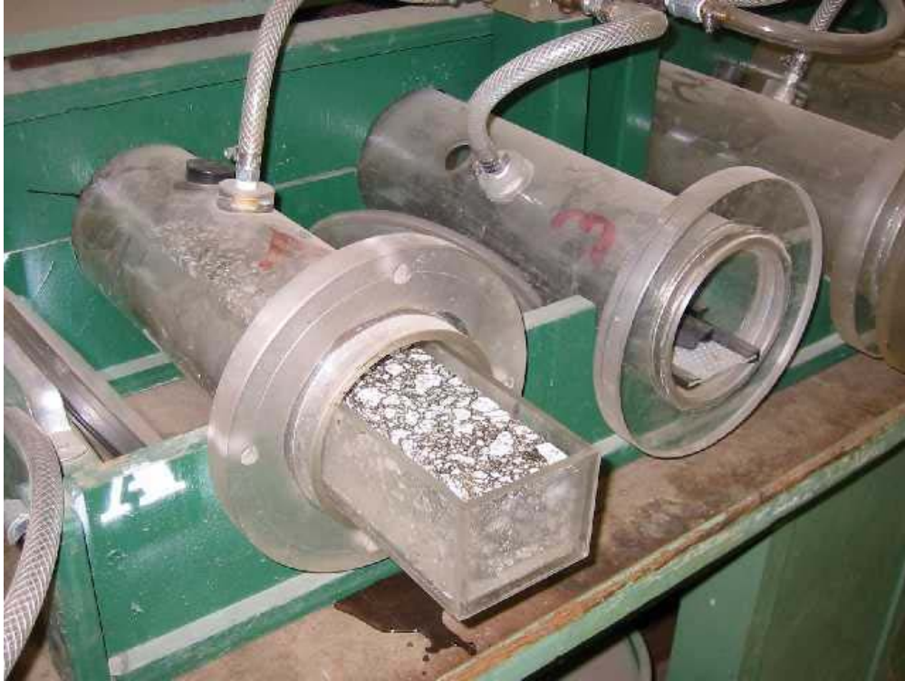
Figure 6-10. Apparatus for saturating specimens by vacuum.
