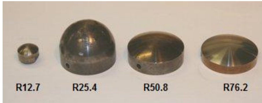
Figure 3. Impact tips of radii 12.7, 25.4, 50.8 and 76.2 mm from left to right
