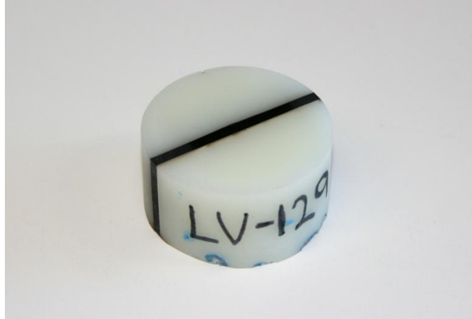
Figure 34. Panel section prepared for microscopy mounted in epoxy
