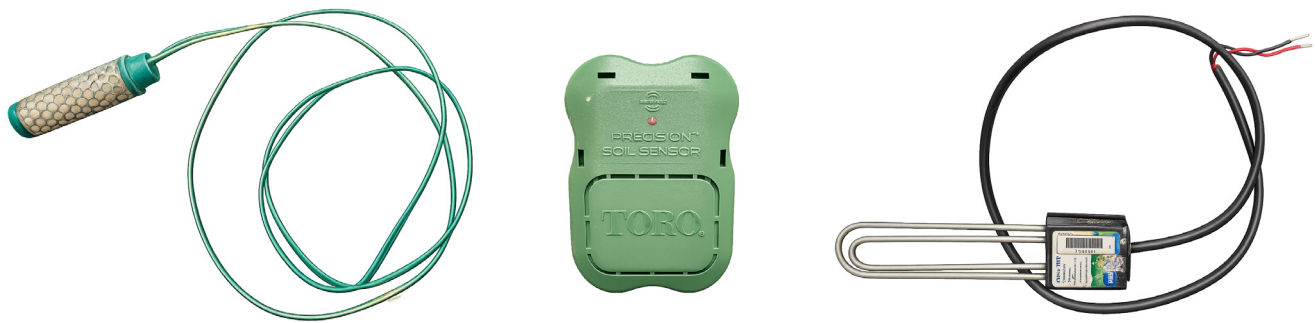
Figure 3. Some commercially available soil moisture sensors: Irrometer Watermark sensor (left), Toro precision soil moisture sensor (center), Acclima digital TDT sensor (right).
