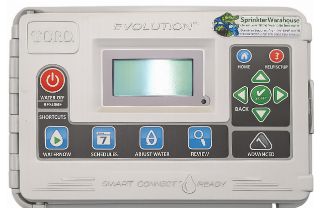
Figure 1. Example of an SMS-based smart irrigation controller. Photo: http://toro.com .
