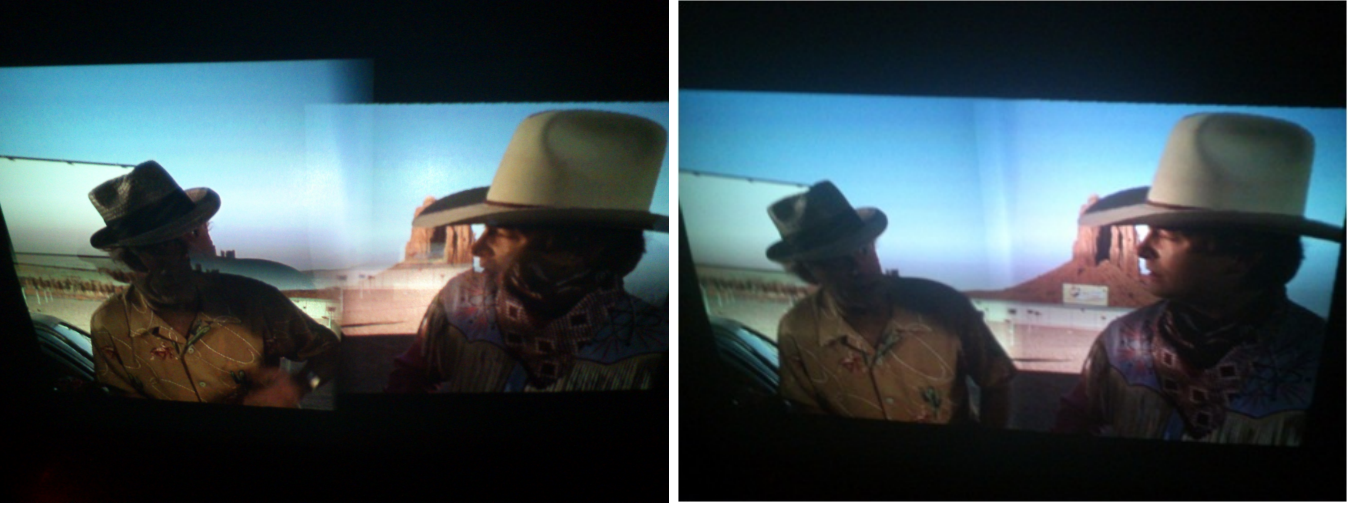
Fig. 7. A collaborative display made of 2 \times 2 array of tiled mobile projectors, before (left) and after (right) registration.
