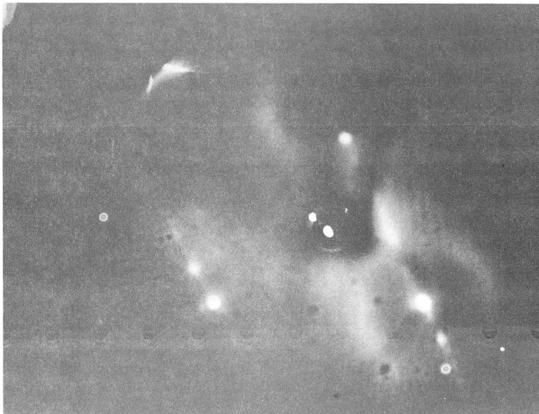
Fig. 6-9. Photograph of LEED pattern from Bz irreversibly adsorbed on the Pt(S)-[6(111)×(100)] surface.
