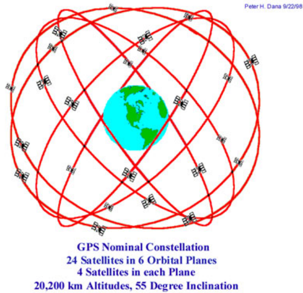
Figure 18: Space Segment of the Global Positioning System [5].
