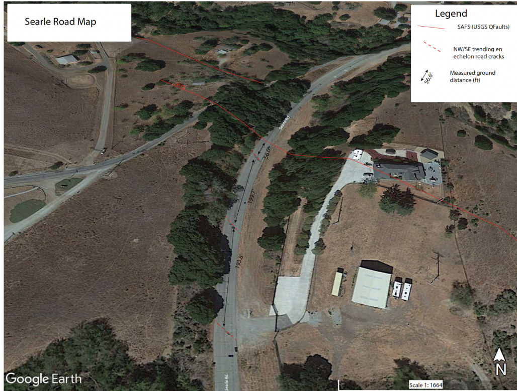
Figure 15. Searle Road site map showing USGS mapped SAF trace in solid red, and three en echelon NW/SE trending road cracks in dashed red lines.
