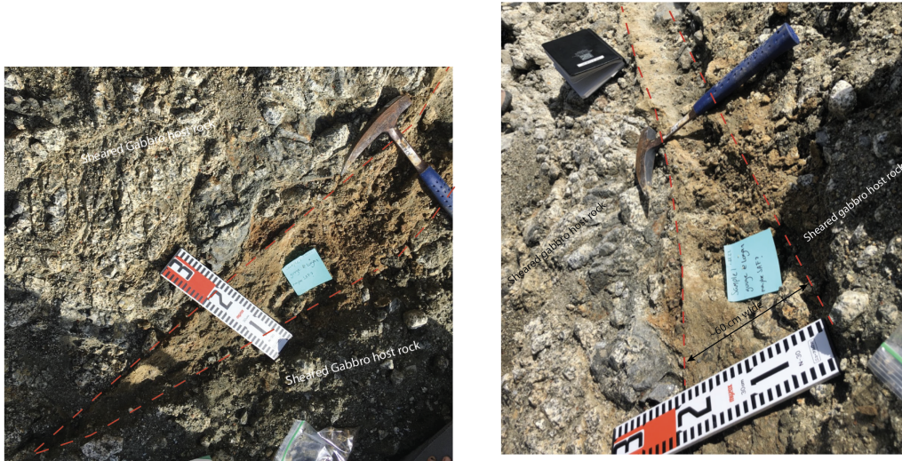
Figure 10.2 Gouge bed located in quarry road floor: fault oriented 090/60 S- 086/61 SE.
