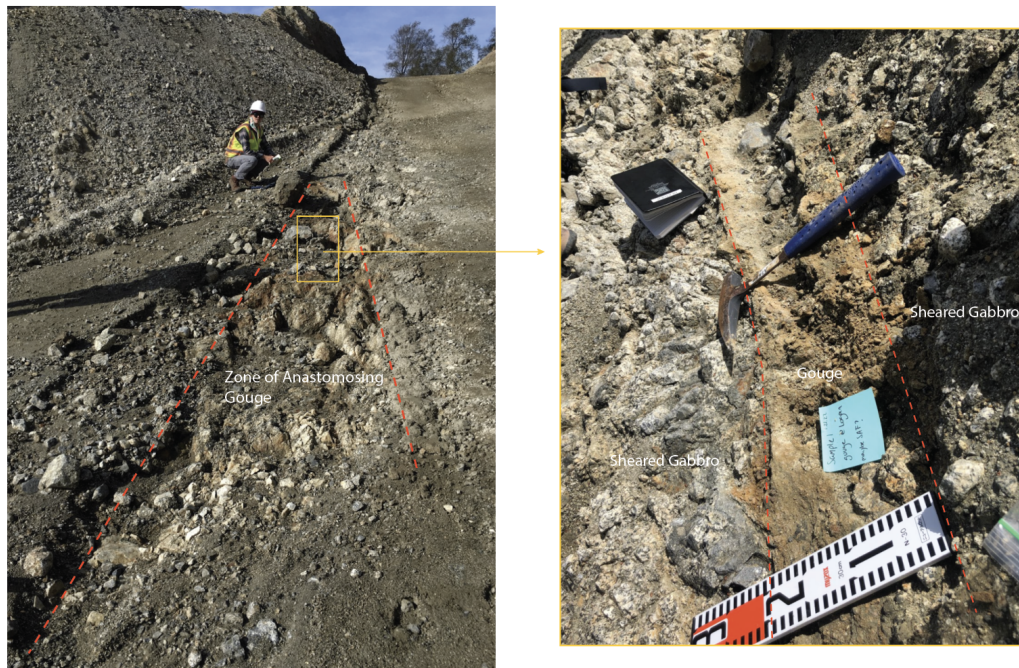
Figure 10.1 Images display anastomosing gouge bed in Logan Quarry road with fault oriented 086/61 SE to 090/60 S. Image on left is an overview image outlining the zone of anastomosing gouge in red dashed lines. Gold colored box outlines area where image on the right is captured. Image on the right depicts the approximate width of gouge bed, with sheared Logan gabbro host rock on either side.
