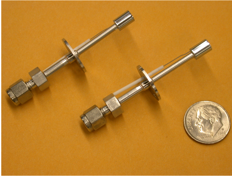
Figure 6.2: MiXI mini cathodes next to a US dime. Cathodes use a BaO insert and have various orifice geometries for discharge and neutralizer operation.
