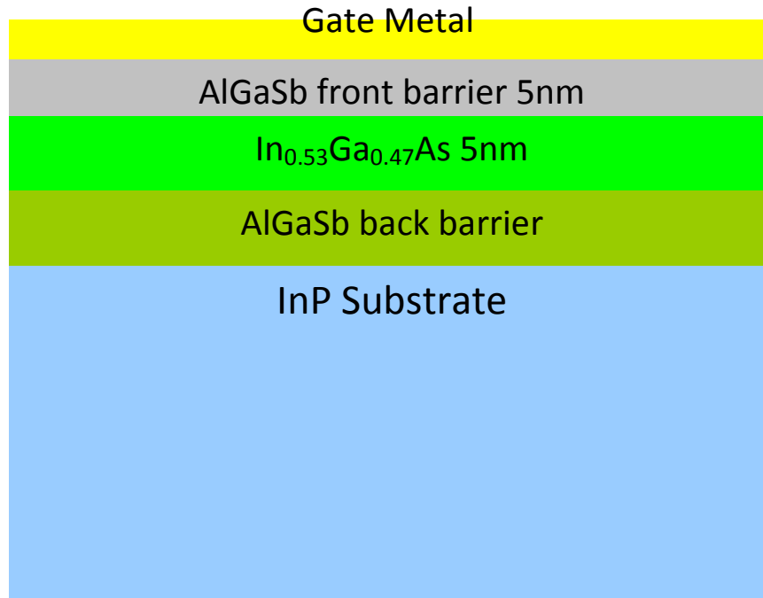
Figure 2.3. Schematic of layer structure computed.
