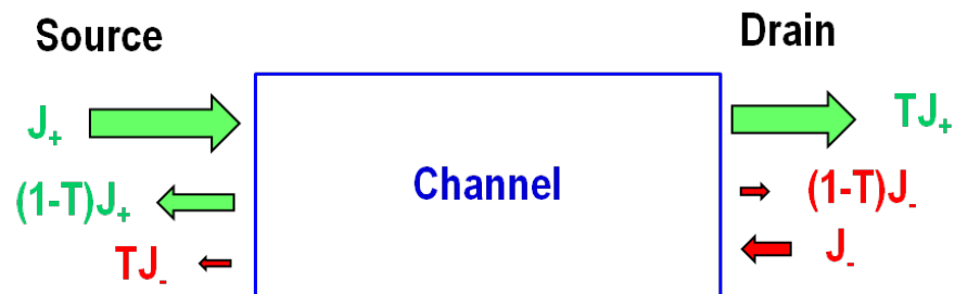
Fig. 3.8. Illustration of the quasi-ballistic transport with the description of transmission coefficient.
