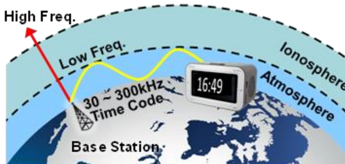
Figure 34: VLF and LF communication is possible over thousands of miles, practically crossing continents.
