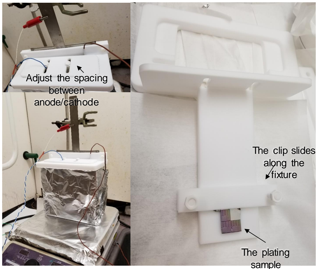
Figure 23: New plating setup. All fixtures are designed and custom made in Teflon. The sample fixture can also support 6" full wafer plating. The new setup better controls the electroplating parameters such as the spacing between cathode and anode; the depth of the sample in the plating solution; uniformity across samples, or even wafers etc.
