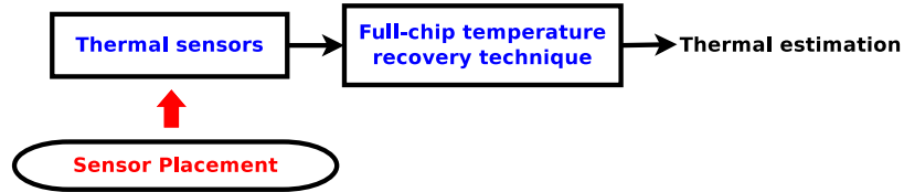
(a) The traditional sensor based thermal estimation flow and the corresponding thermal sensor placement.
