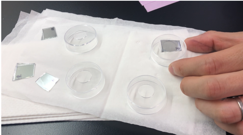
Figure 1.3: The mirrors are cut into 2 \times 2 mm pieces and glued to bottomless cell culture dishes
