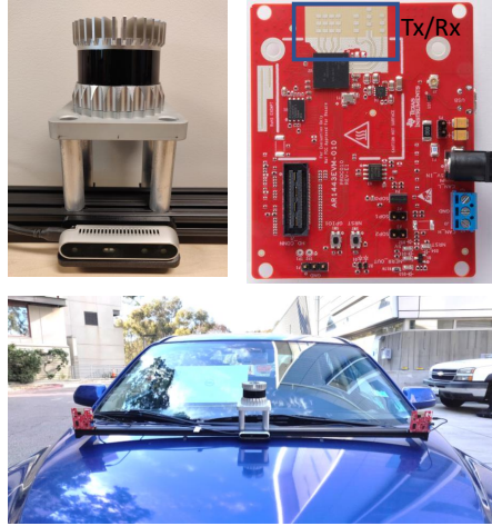
Figure 1.12. Pointillism data collection platform. (Top Left) 16-channel Ouster LiDAR, RealSense Depth Camera for ground truth labels. (Top Right) our radars. (Bottom) Our System: Two radars, LiDAR, Depth camera combined synchronously to common clock.
