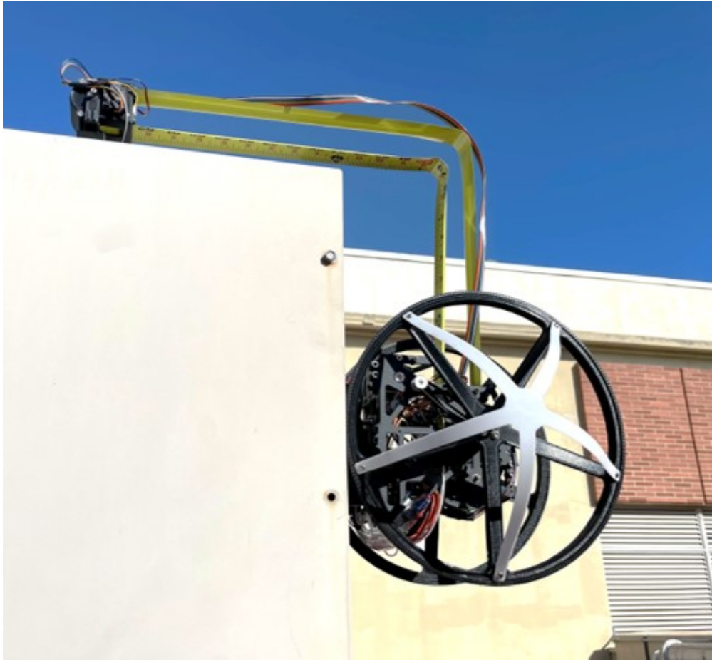
Figure 4.21: EEWOC bending its limb to place its gripper on top of a 90° ledge.
