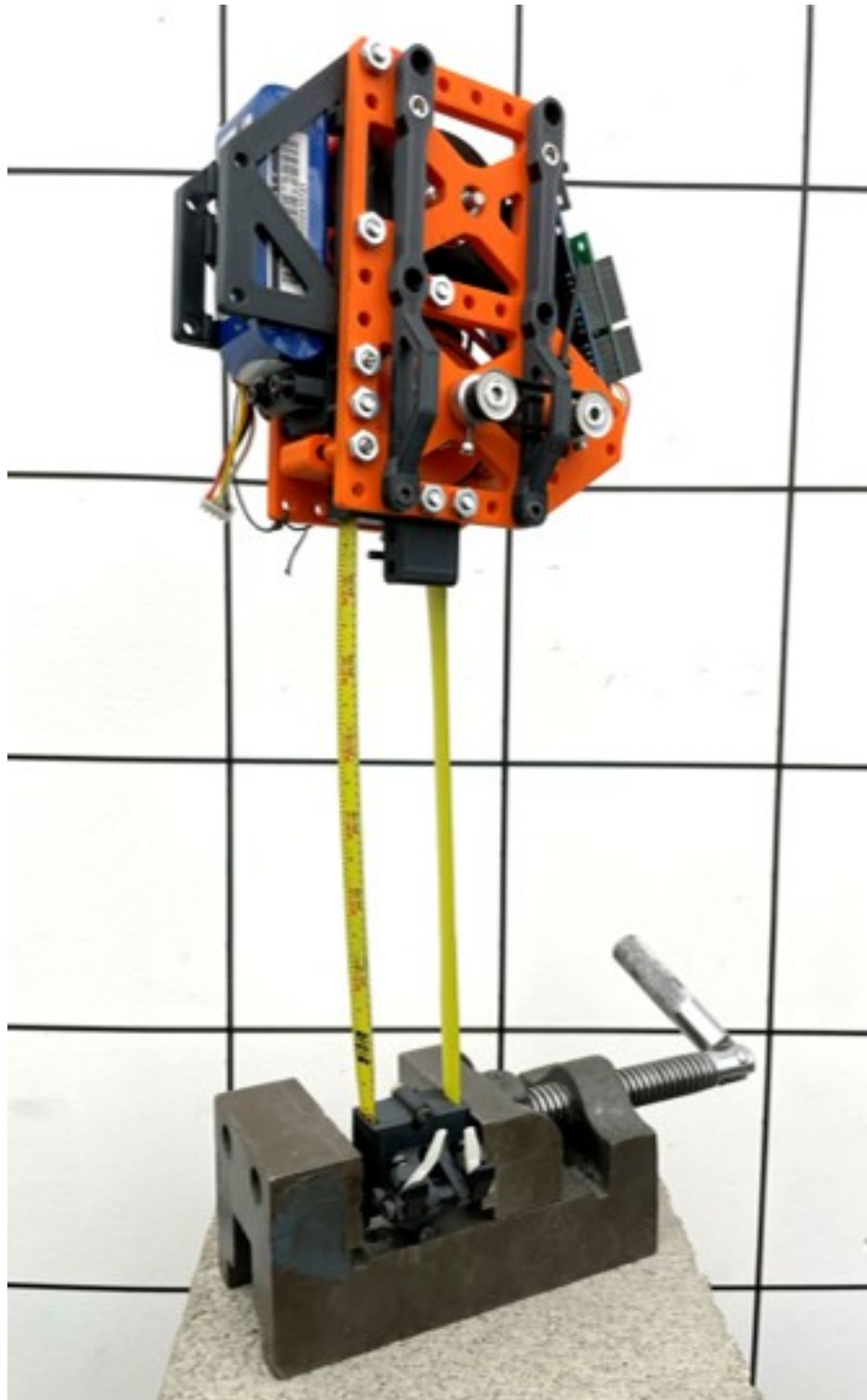
Figure 3.12: EEMMMa standing demonstration. The limb is deployed downward, with the end effector secured in a vice. The weight of the main body loads the limb in compression, similar to a weight-bearing leg.
