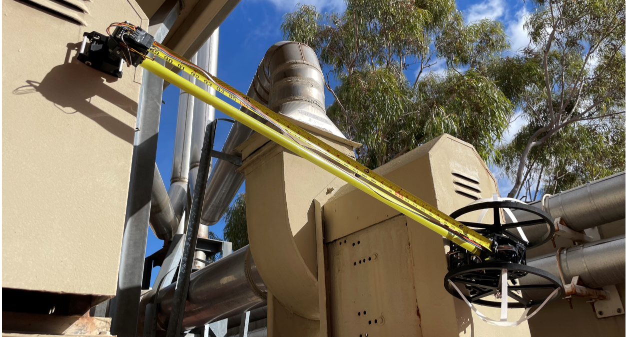
Figure 4.18: EEWOC straight sideways deployment demonstration. This can be useful for traversing gaps or moving between distant features.
