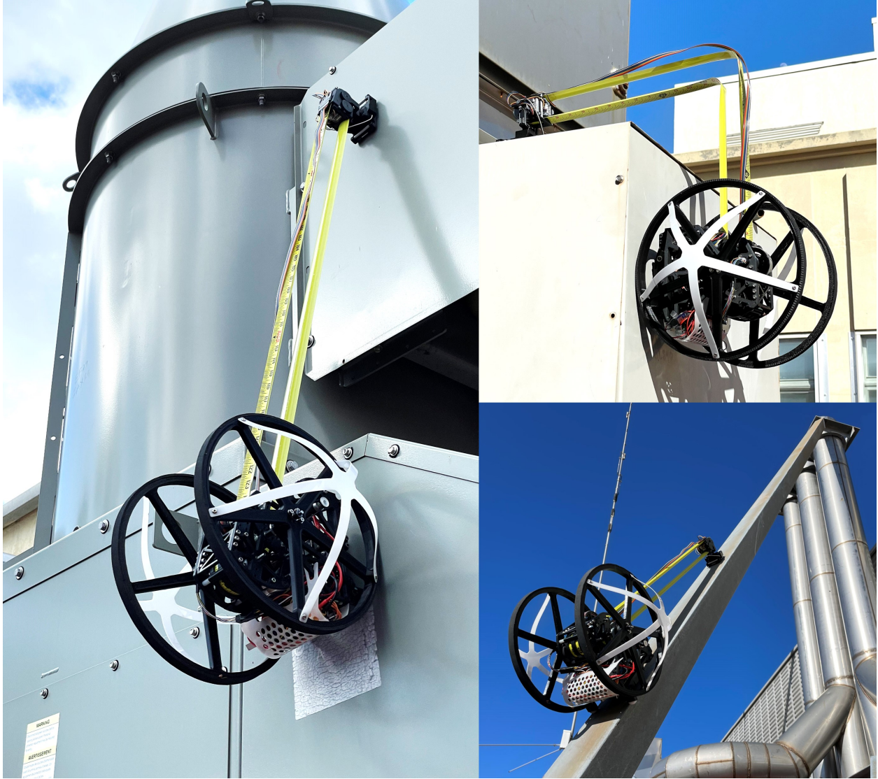
Figure 1.3: EEWOC's ability to extend and bend to place its magnetic grippers on complex features grants it a wide variety of mobility options on steel structures. Here, it is shown extending over a small gap on HVAC machinery, bending to reach the top of a ledge, and climbing up a tall support truss.
