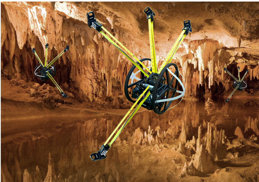
Figure 5.4: Concept art of future EEWOC units in a cave, suspending with microspine grippers to traverse over water and rocky terrain.
