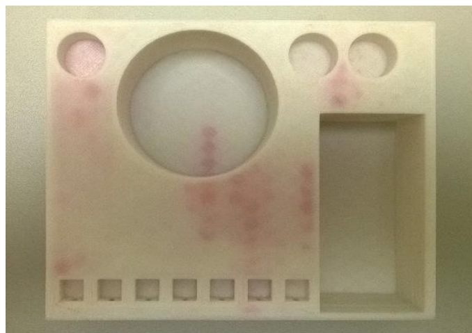
Figure 8: Printed part with leakages showing red. Dyed water marks the hexagonal infill structures filled with water through leakages from chambers and enclosed channels into the part.
