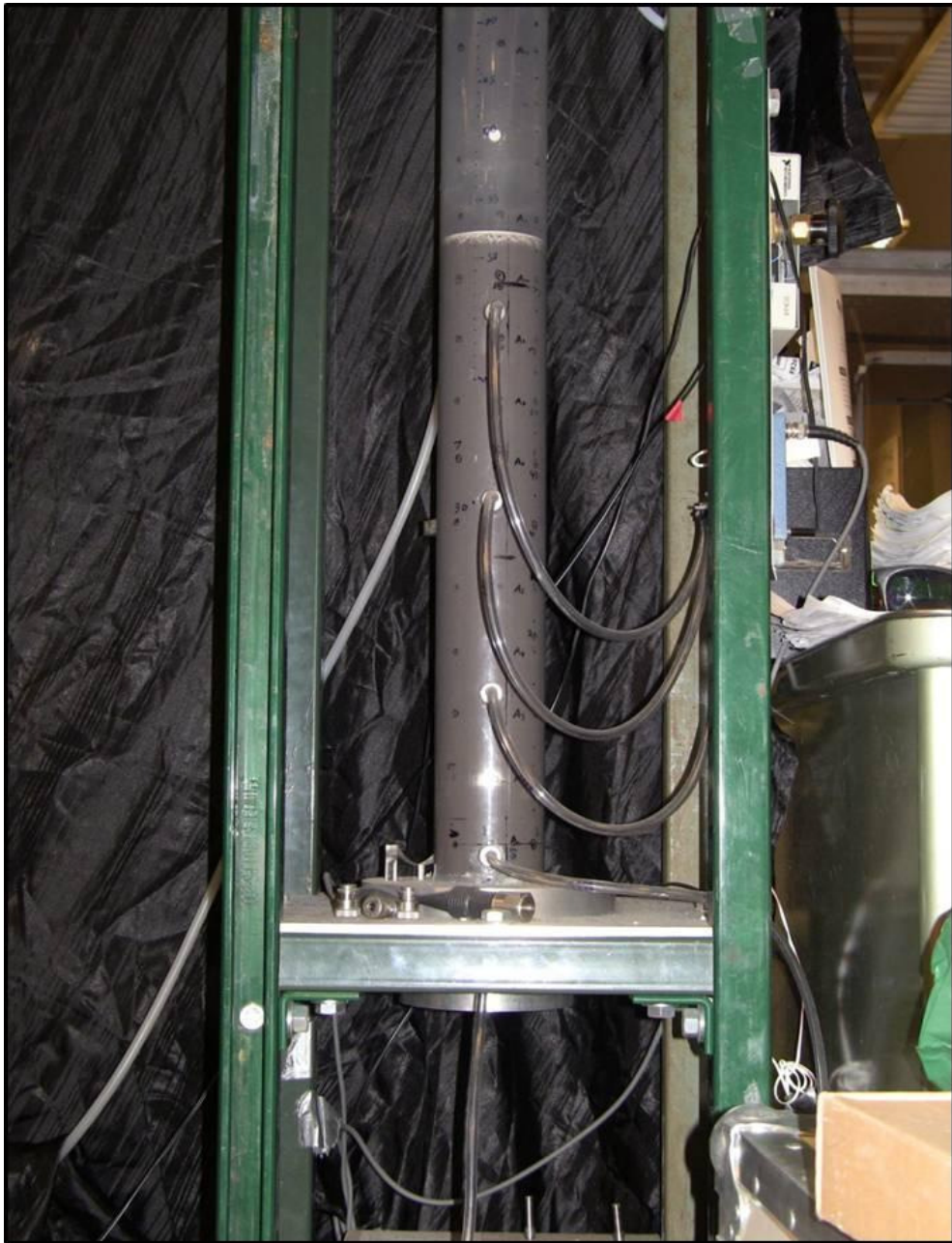
Figure 8.2: Photograph of the vertically-oriented fluidized bed experiment. Tubes connected to the pressure taps converge on the signal conditioning and amplification circuit, which is not visible.
